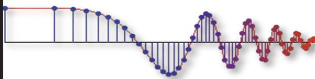
The explosion sound wave is transformed into a sequence of samples.
