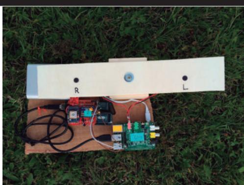
First Sensing Node prototype during outdoor field test campaign
