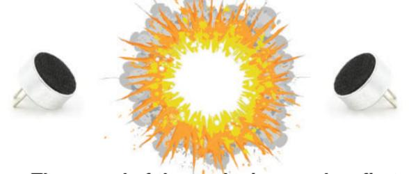
The sound of the explosion reaches first the closest microphone.
